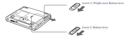
2 After removing the weight saver, pull out the weight saver's hinged arm and fold it into the weight saver.
